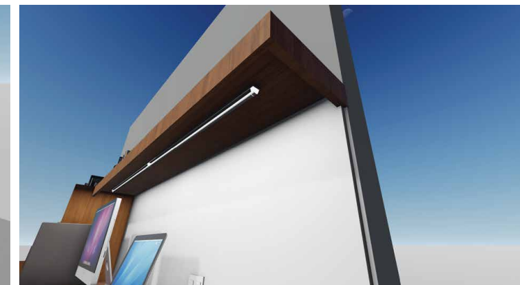
Placement of light shown, It is turned off/on with switch on front wall
