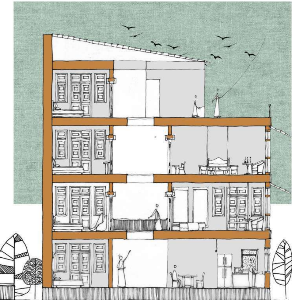
Section DD _Showing the courtyard that gives in diffuse light to create a holistic shine to the Pooja place.
