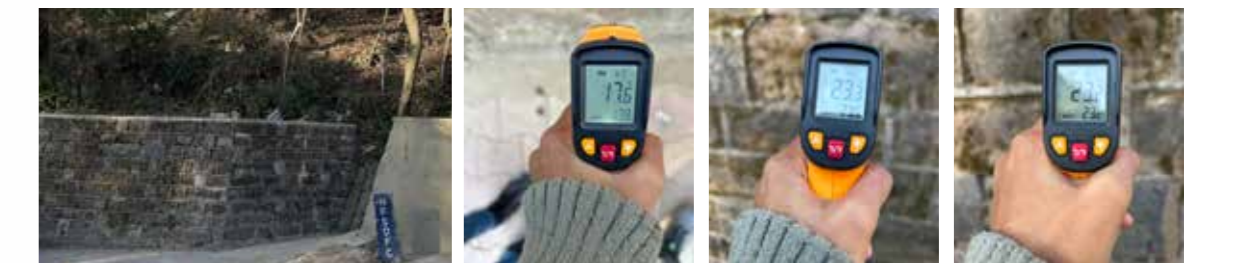
Measuring the temperature of different portions of a South facing stone wall Lower stone wall: 17.6 °C Middle stone wall: 23.3 °C Upper stone wall: 23.2 °C
